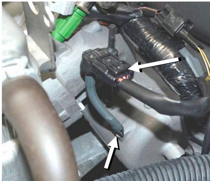
Under map sensor disconnect vacuum hose from intake manifold.
