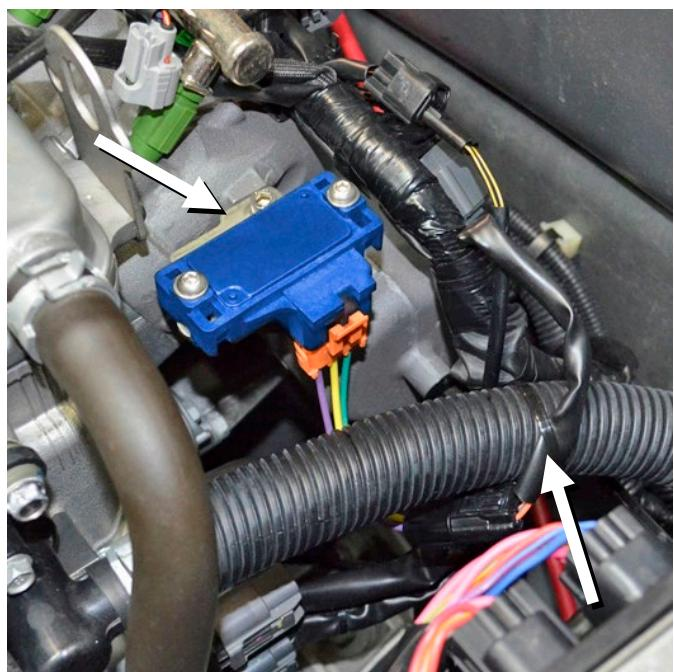
Connect open end of map sensor wire to wiring harness. Secure to cooling hose using supplied large zip tie.
